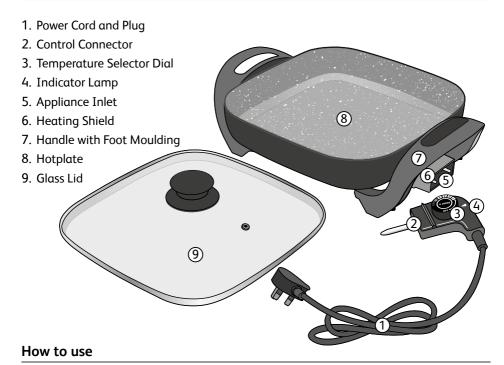
Before Operation: insert the Control Connector ② firmly as far as it will go into the Skillet's Appliance Inlet ⑤, leaving the Temperature Indicator ③ set below the Minimum mark - turn it anti-clockwise as far as it will go. Then insert the Power Cord Plug ① into the mains socket. (The Electric Frypan may emit abnormal smells when used for the first time - they are not hazardous and will disappear after a few minutes). When cooled wipe the hotplate with a damp cloth.
