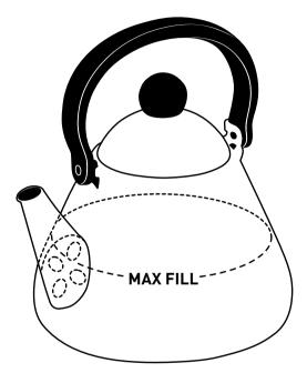
WHEN FILLING, NEVER ALLOW WATER TO COVER THE TOP HOLE.
